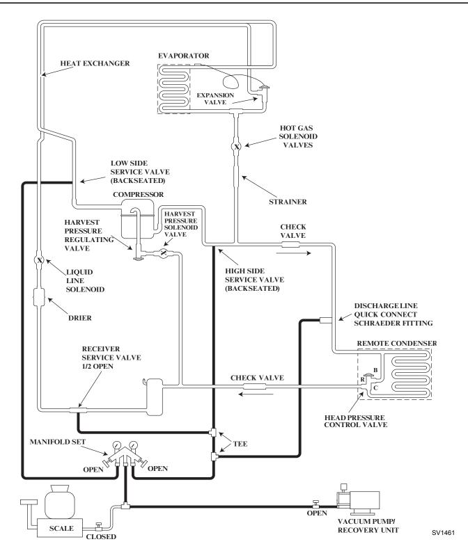
Figure 7-9. Recovery/Evacuation Connections
